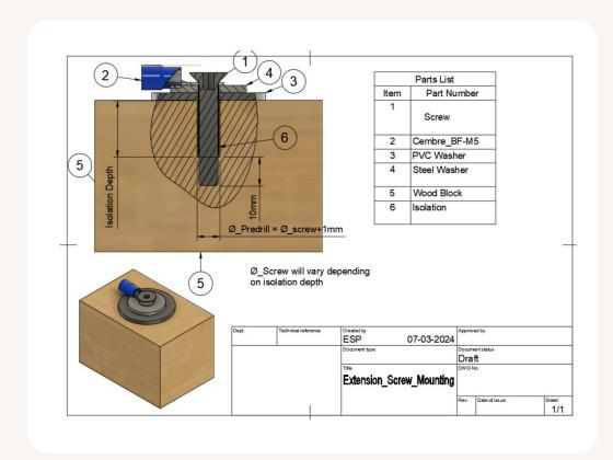
If you have insulated pins AND an extension, it's important to remember the accompanying washers in between the extension and the timber to prevent surface readings.
