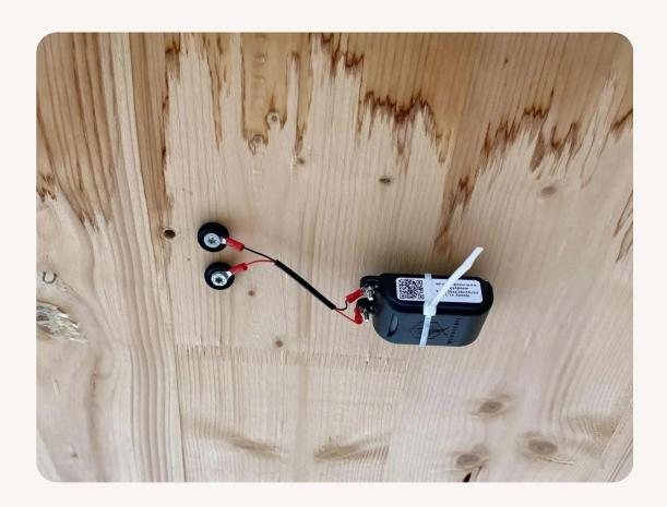
This can be useful if the extension is measuring in a CLT roof element from below or if the sensor casing needs to be attached to a column, while the wood moisture reading is elsewhere.
