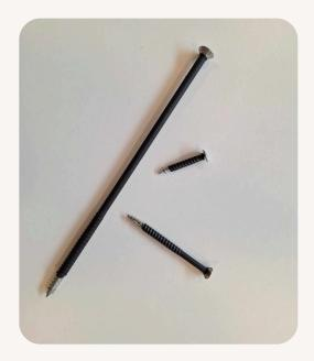
You want to insulate the pins, when you want to measure the wood moisture content at a specific depth or want to avoid high spikes in moisture readings caused by rain and water on the surface of the timber. Without insulated pins, the sensor will measure the wood moisture content, where the moisture is the highest between the two pins.
