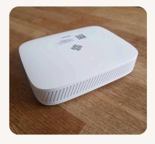
Plug the gateway into power and find a location where the signal is not deflected and where the gateway will not be unplugged in the future.
